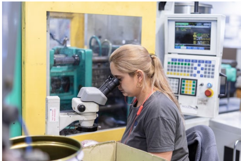
Fig. 5 Visual quality inspection of MIM parts (Courtesy CMG Technologies)
