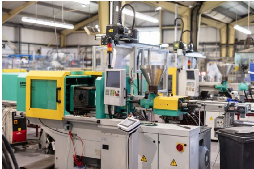
Fig. 4 An Arburg injection moulding machine with a robotic system for the removal of parts from the mould (Courtesy CMG Technologies)
