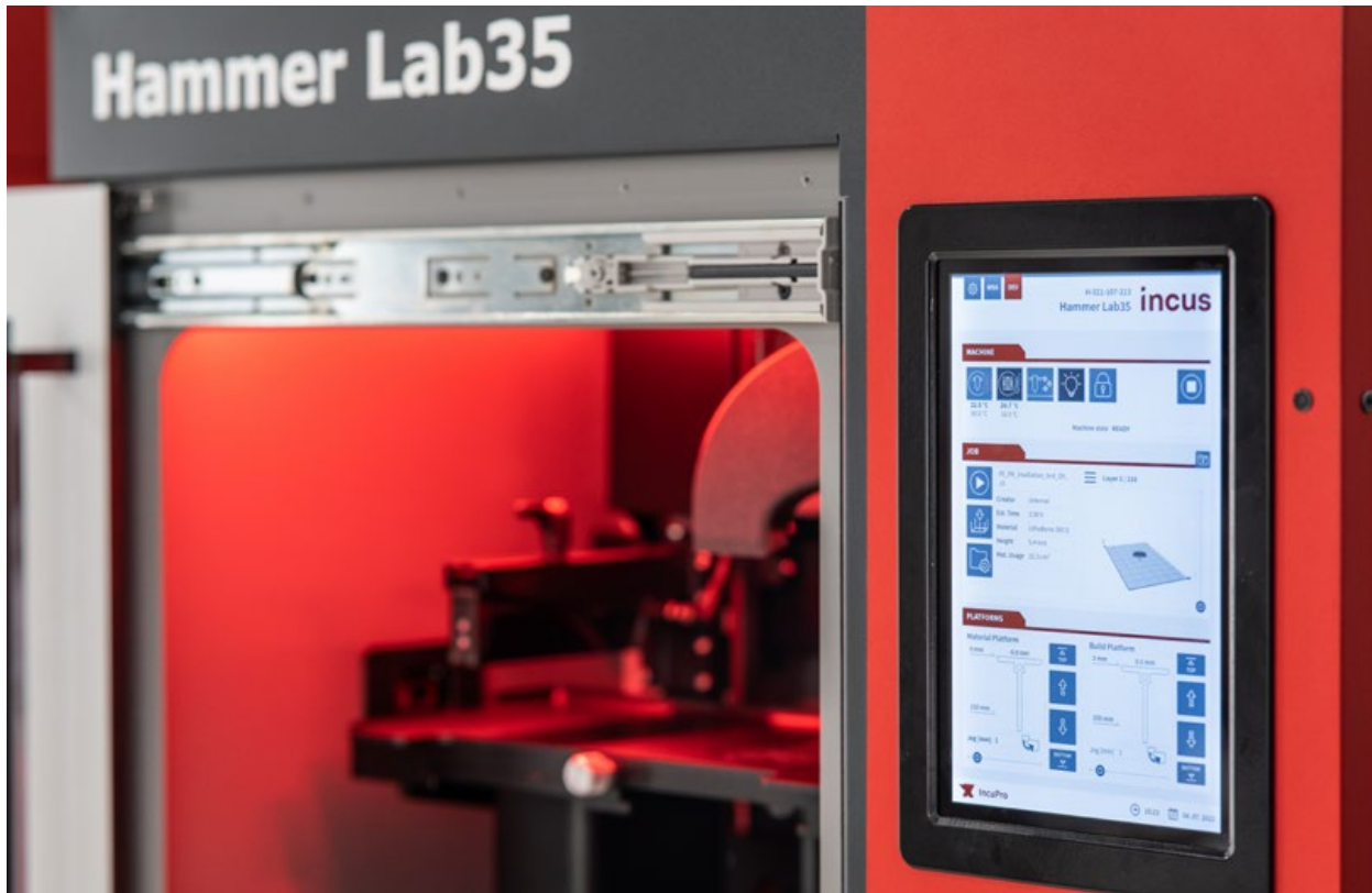
Fig. 4 Incus' Hammer Lab35 AM machine is capable of producing parts with mechanical performance and surface finish that is equivalent to Metal Injection Moulding (Courtesy Incus GmbH)
