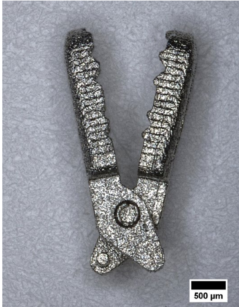
Fig. 14 A laparoscopic tool mini-gripper produced by Vat Photopolymerisation (Courtesy Incus)
