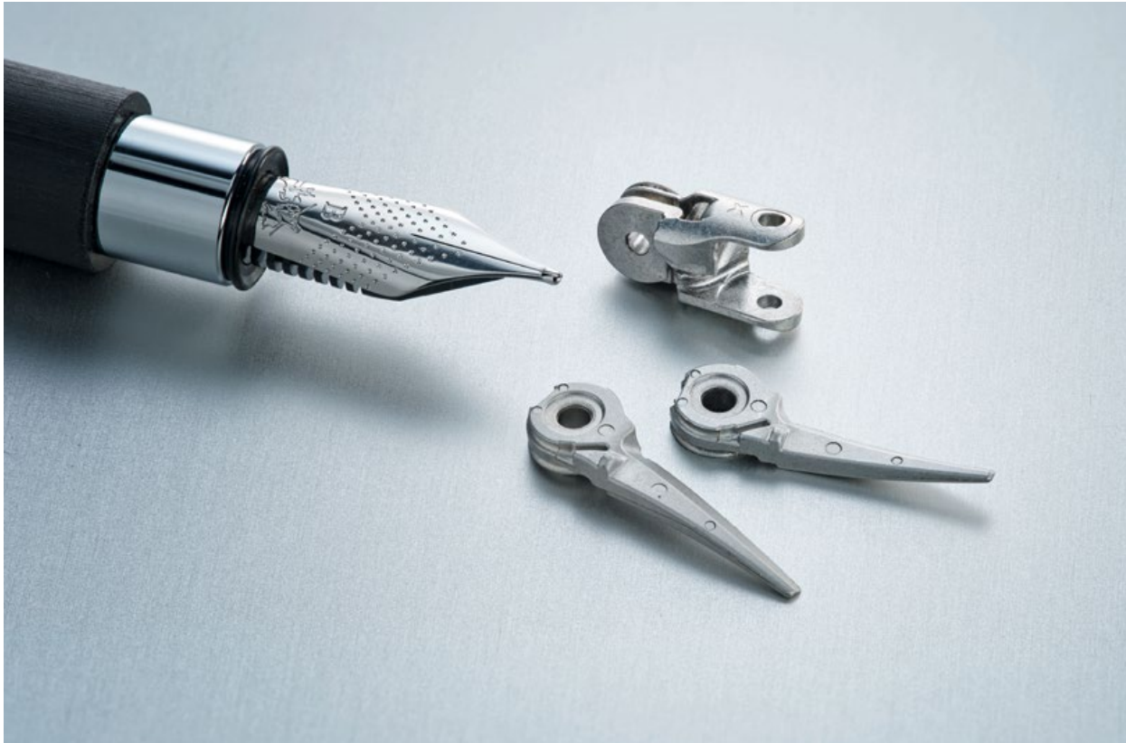
Fig. 10 The tip core (upper part) is an articulated piece of an instrument control system for robot-assisted surgery, made from 17-4 PH stainless steel. The lower parts form a pair of scissors that are used as a cutting instrument in robot-assisted surgery and are made of AISI 420 martensitic stainless steel (© 2023 Distalmotion. Image used with permission)
