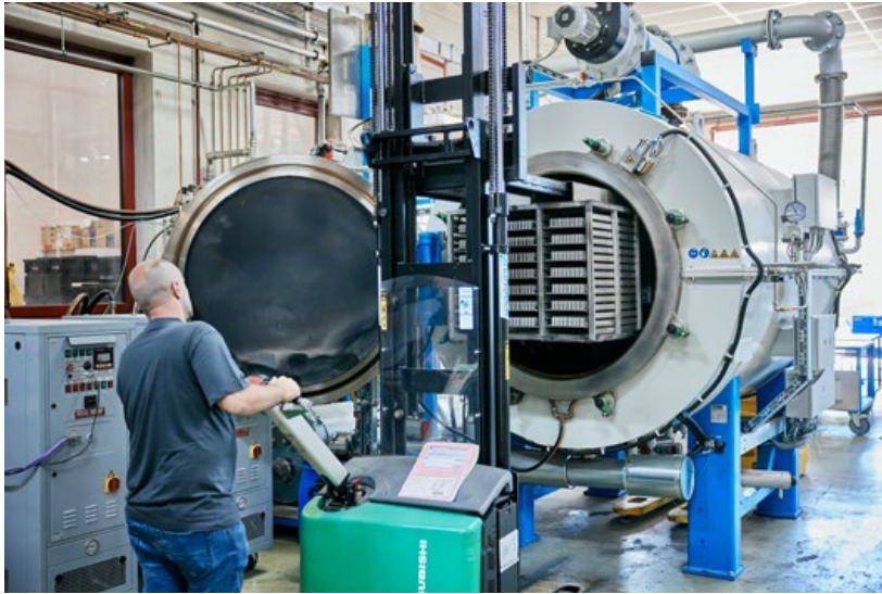
Fig. 2 A batch of green MIM parts being loaded in a furnace (Courtesy Parmaco)
