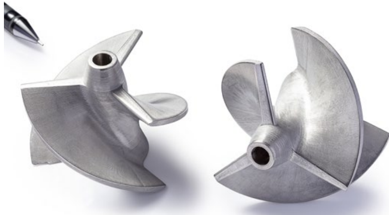
Fig. 13 A 17-4 PH stainless steel propeller manufactured by MEX/FFF from CMG Tech-X filament and used in Safety Of Life At Sea (SOLAS) boats (Courtesy CMG Technologies)
