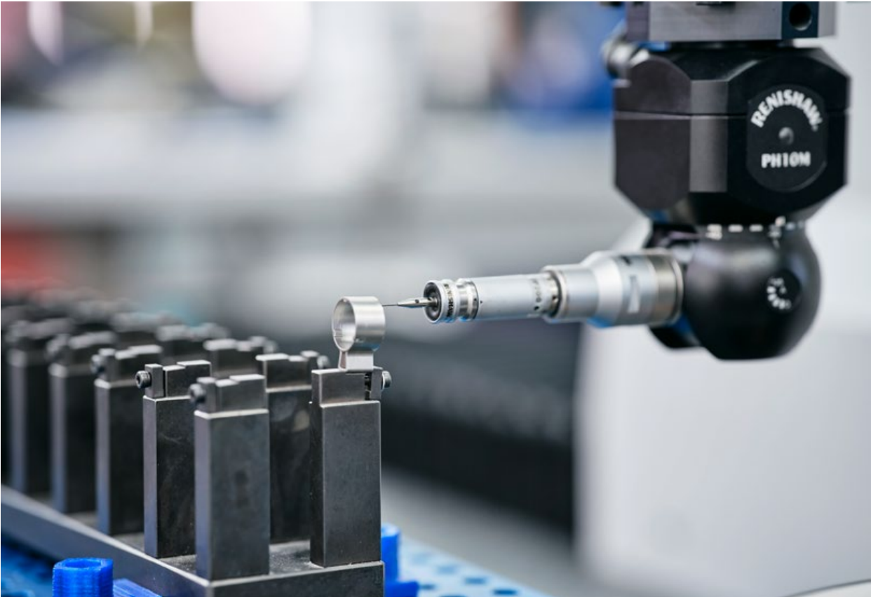
Fig. 4 Precision measurement of part dimensions (Courtesy Parmaco)
