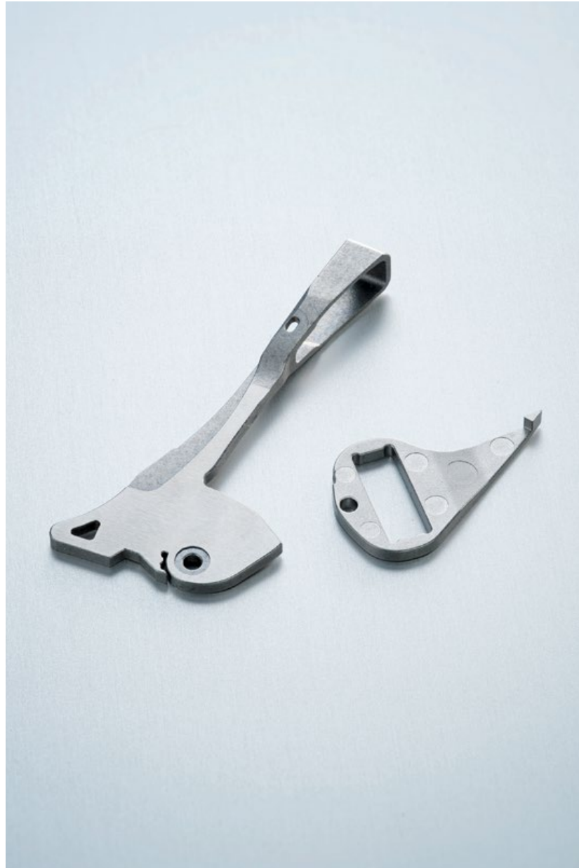
Fig. 9 These inserts are critical control components in vessel sealing instruments. The part is overmoulded with thermoplastic and serves as a lever for actuating the vessel seal. This insert is made from 17-4 PH stainless steel (Courtesy Parmaco)
