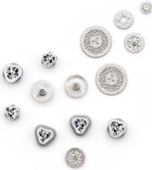
Fig. 3 As-sintered parts designed by Leap 71 and additively manufactured with Incus' Hammer Lab35 AM machine (Courtesy Incus GmbH)
