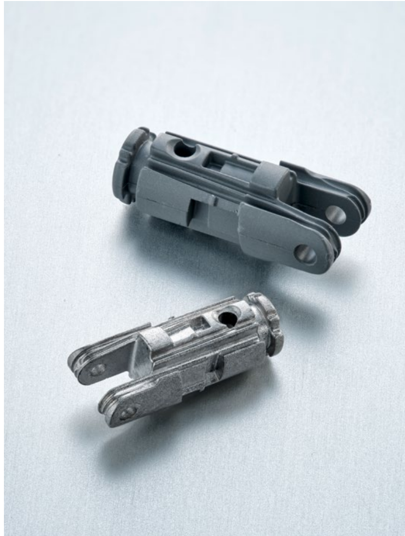
Fig. 11 This fork is an articulation part used in the instrument control system of a robot-assisted surgical device. It is made of 17-4 PH stainless steel and is shown in the green and as-sintered states (© 2023 Distalmotion. Image used with permission)
