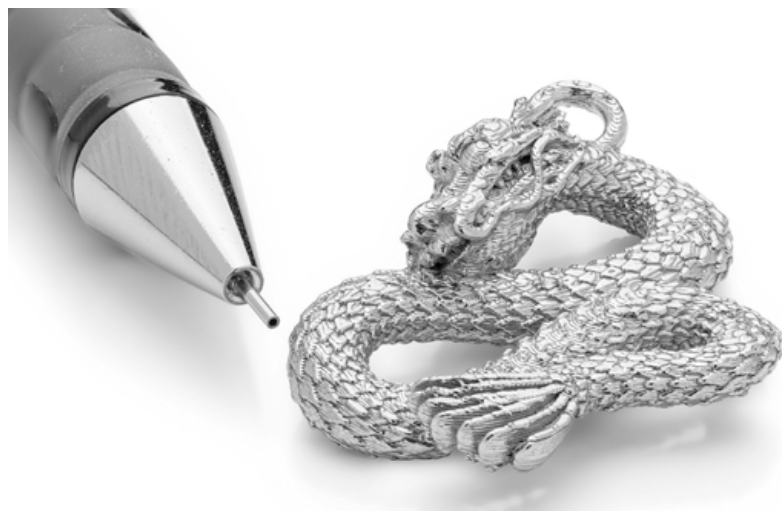
Fig. A 17-4 PH stainless steel decorative part manufactured by MEX/FFF from CMG Tech-X filament (Courtesy CMG Technologies)
