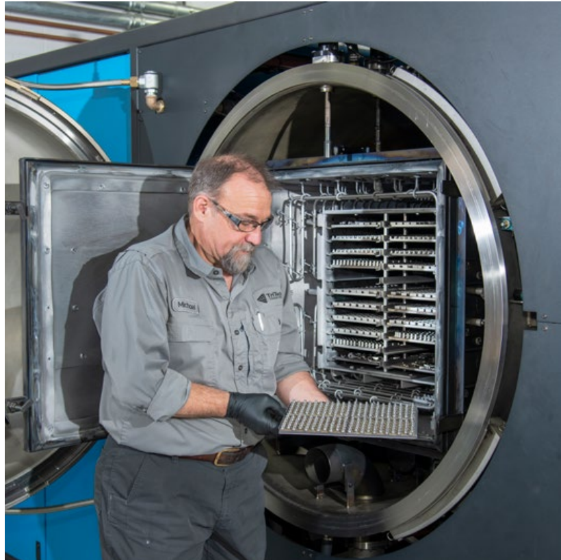
Fig. 3 A tray of sintered titanium parts being removed from an Elnik Systems vacuum sintering furnace (Courtesy TriTech Titanium Parts)
