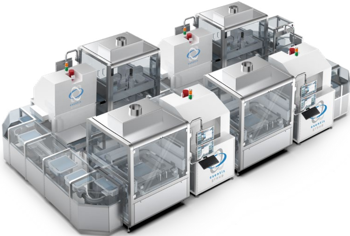
Fig. 4 An Exentis clean room production system for the mass production of tablets with four printing units and four drying units (Courtesy Exentis Group AG)
