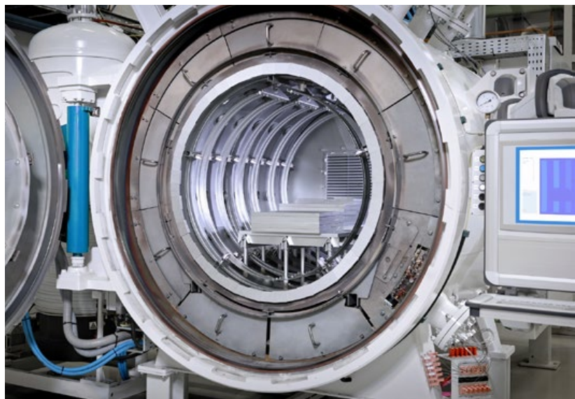
Fig. 1 This vacuum sintering furnace, installed at Plansee Group, Reutte, features numerous energy-saving innovations (Courtesy Plansee SE)
