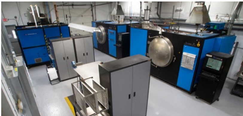
Users of Tritone's MoldJet sinter-based AM technology will have access to DSH's sintering furnaces and expertise (Courtesy DSH Technologies)
