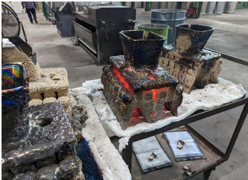
Fig. 11 Investment Casting moulds cooling (Courtesy TriTech Titanium Parts)
