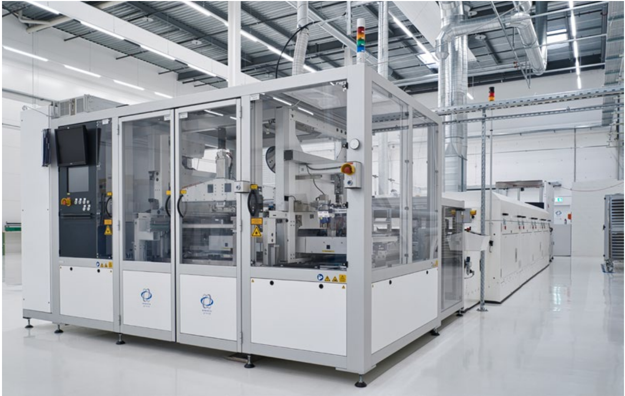
Fig. 5 Exentis' production system suitable for industrial mass production with one printing unit (foreground) and a long drying unit (background) (Courtesy Exentis Group AG)
