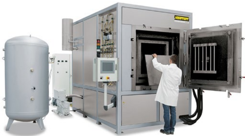
Nabertherm offers a range of furnaces for the heat treatment of metals, including cold-wall retort furnaces for sintering (Courtesy Nabertherm GmbH)
