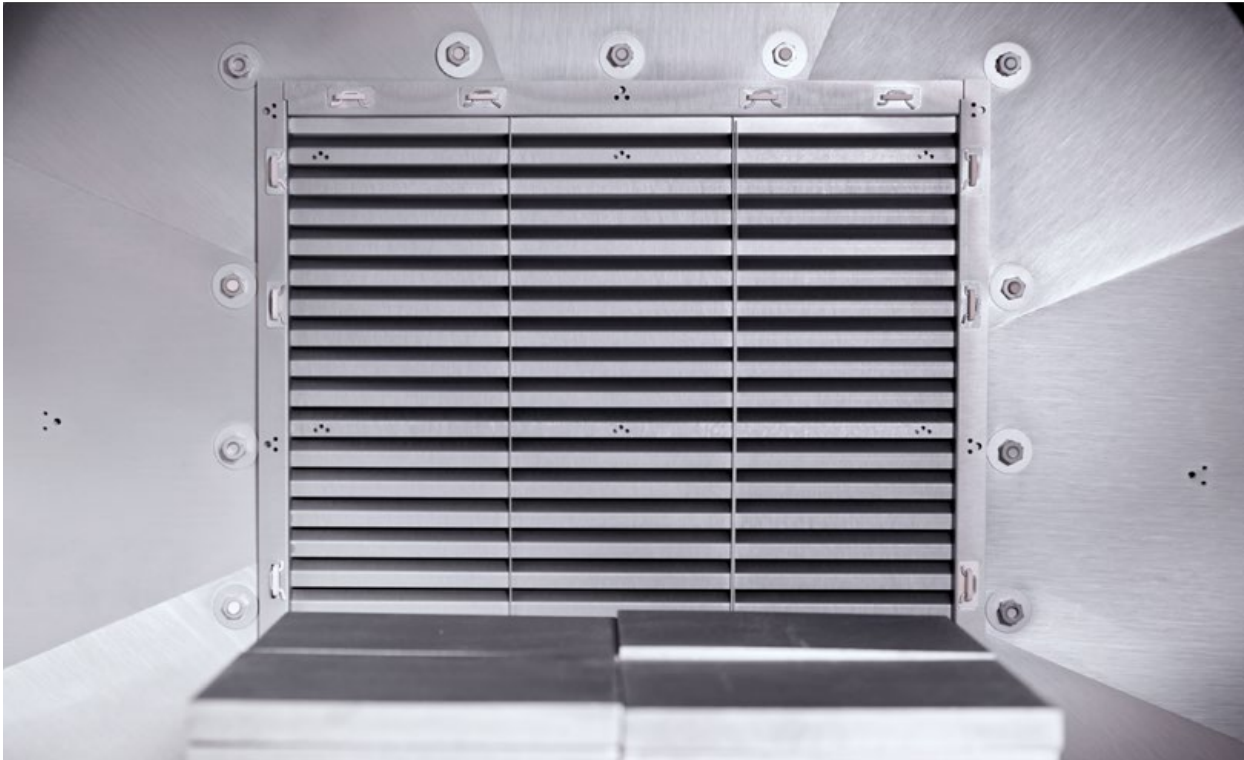
Fig. 5 The patented FlowBox gas outlet, integrated into the rear shield (Courtesy Plansee SE)
