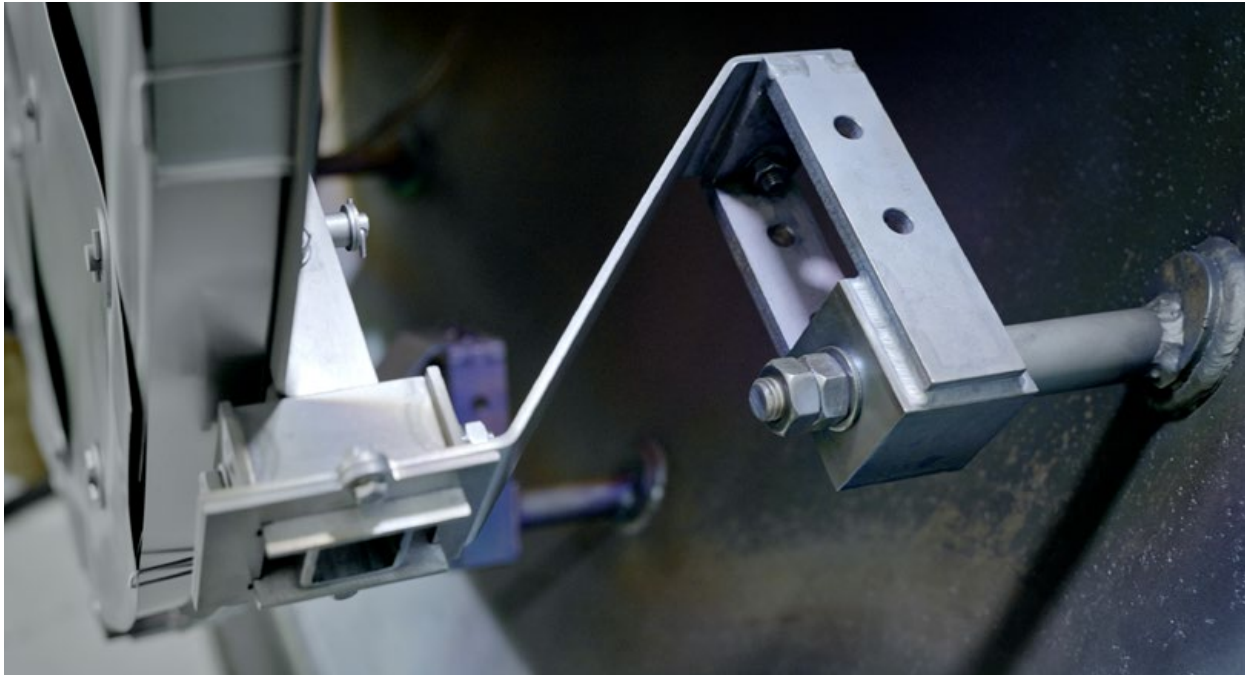
Fig. 7 Patented flexible fixture of the front door with automatic gap control (Courtesy Plansee SE)
