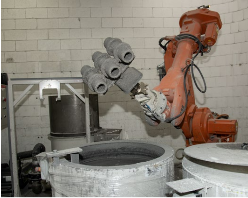
Fig. 10 A robotic arm preparing to dip an Investment Casting mould into slurry (Courtesy TriTech Titanium Parts)
