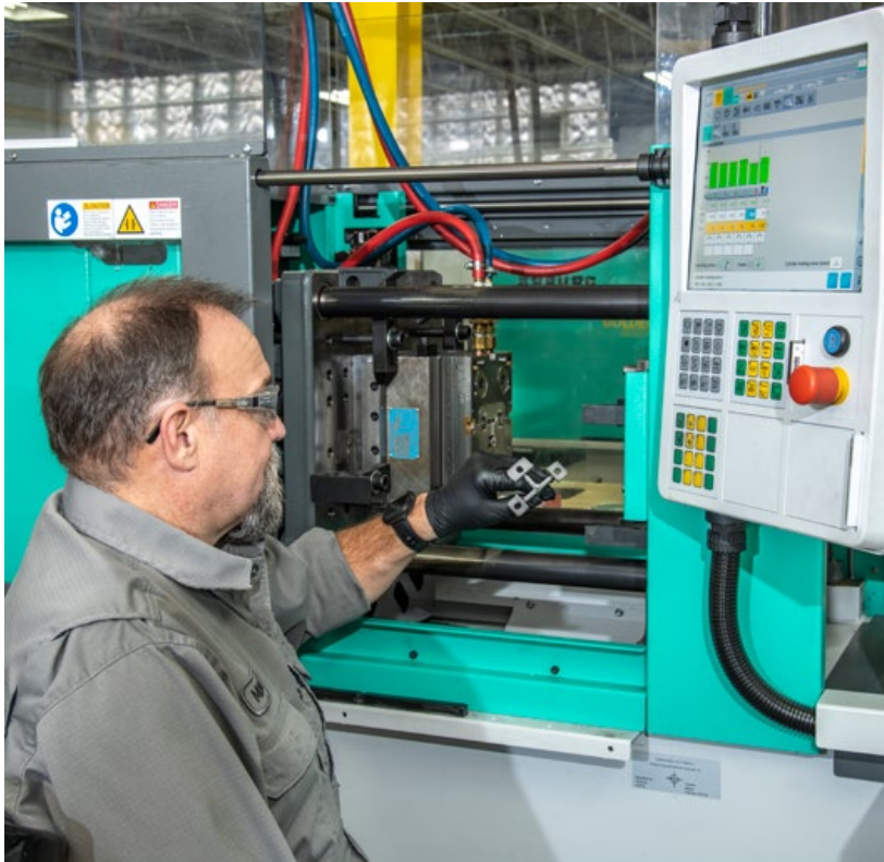
Fig. 4 Parts being removed from an Arburg Allrounder injection moulding machine (Courtesy TriTech Titanium Parts)
