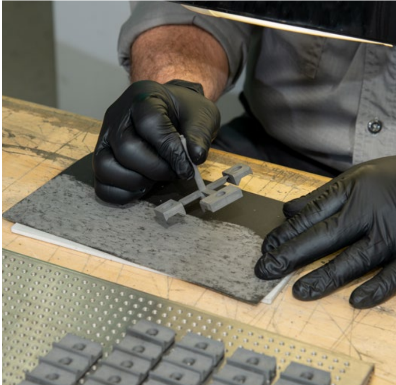
Fig. 5 Parts are removed from the sprues (which are recycled into feedstock) and then placed on perforated stainless steel trays in readiness for solvent debinding (Courtesy TriTech Titanium Parts)
