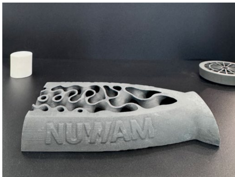
Fig. 1 A silicon carbide gyroid structure on display at Ceramitec 2026, manufactured by NUWAM using D3 Additive Manufacturing's Binder Jetting technology (Courtesy D3)
