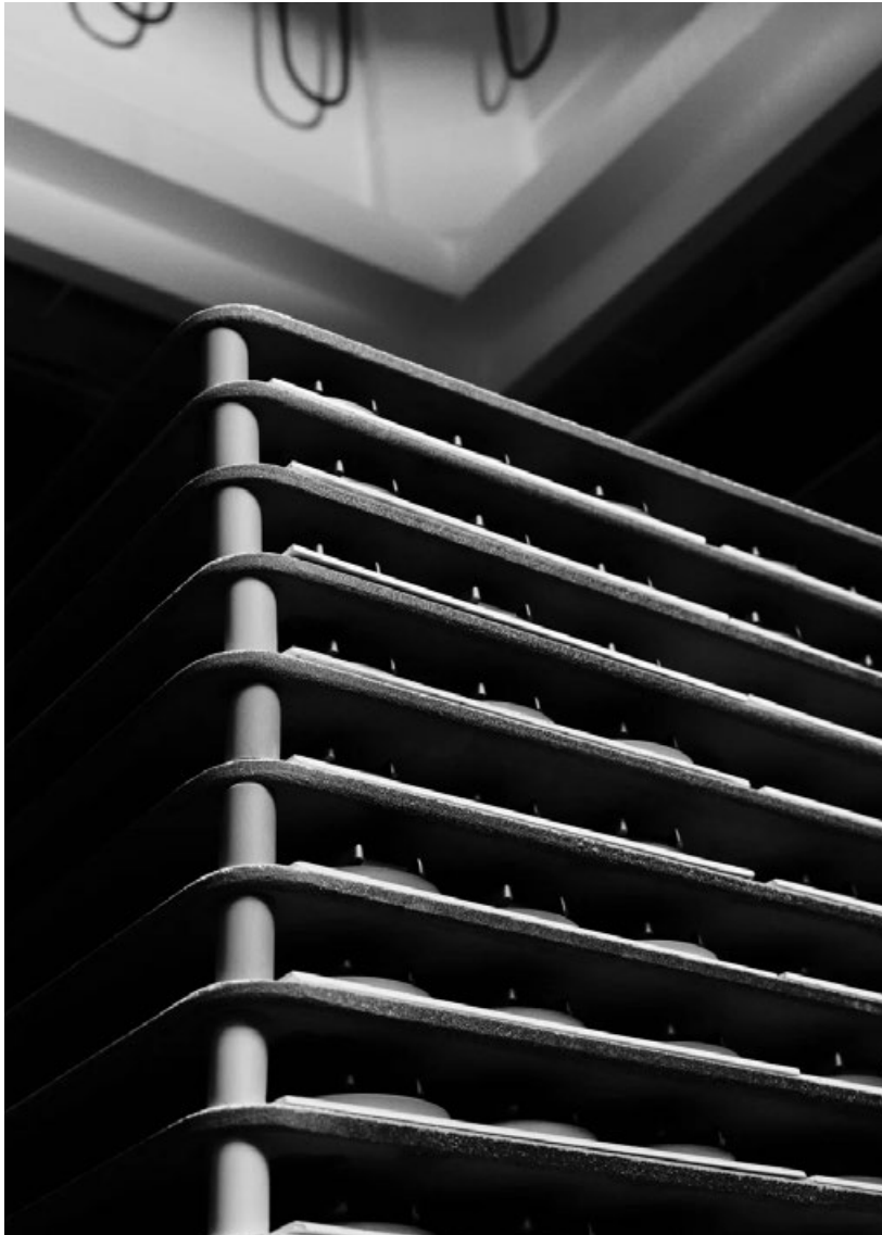
Fig. 8 Sintering trays beneath a furnace (Courtesy Chanel)
