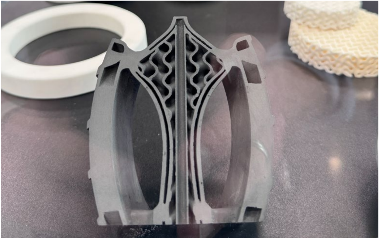
Fig. 16 A ceramic aerospike rocket-engine cutaway presented by D3 Additive Manufacturing at Ceramitec 2026 (Courtesy Nick Williams/PIM International)
