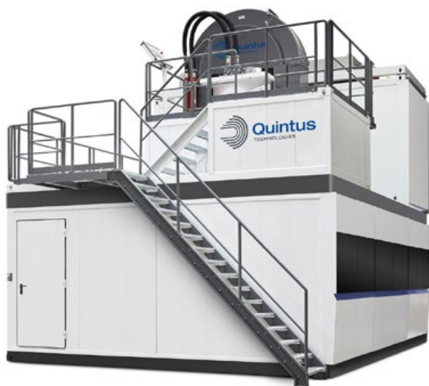
Fig. 10 Quintus Technologies Hot Isostatic Press (HIP) (Courtesy Quintus Technologies)
