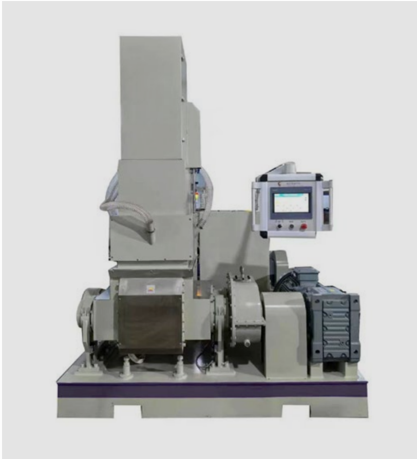
Fig. 8 High-capacity feedstock mixing machine for MIM production, capable of processing approximately 200 kg of SUS 304 feedstock per batch, with mixing completed within ~1 hour (Courtesy Dongguan Changfeng Machinery (C-Fine) Technology Co, Ltd)
