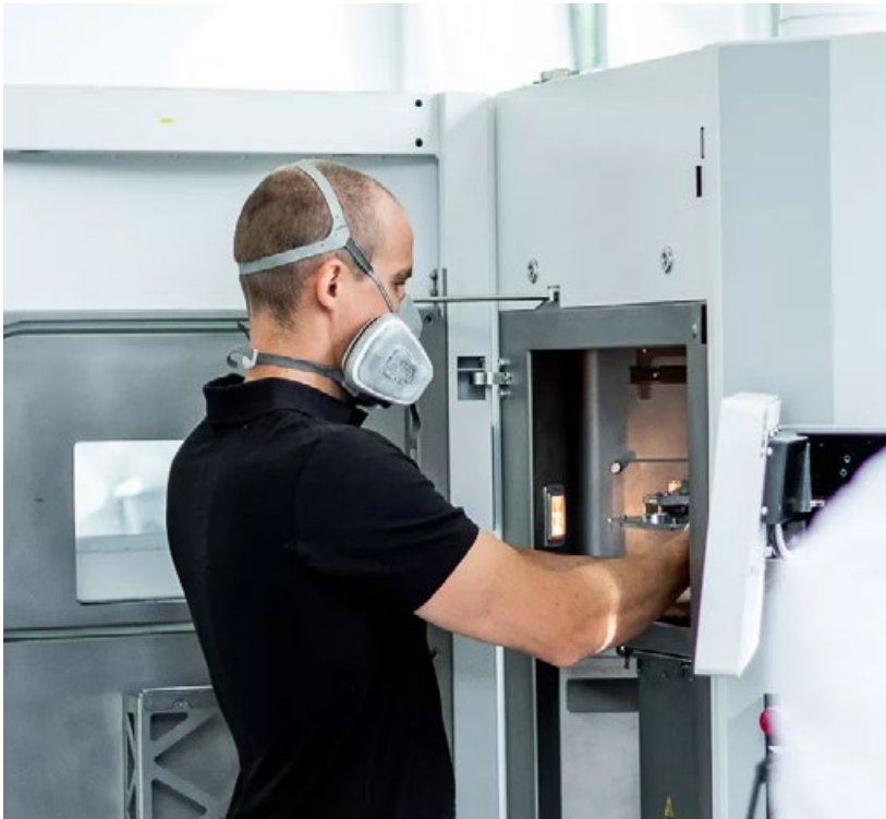
Fig. 9 Operator working with a polymer PBF-LB machine (Courtesy Headmade Materials)
