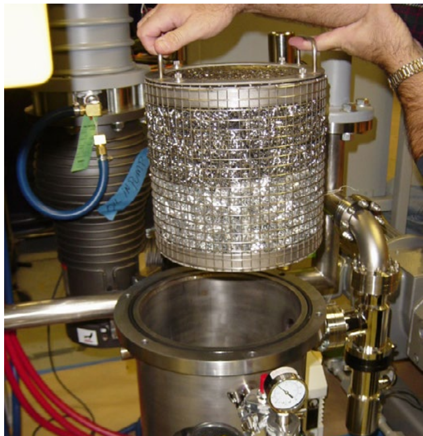
Fig. 9 Example of a binder trap (Courtesy Centorr Vacuum Industries)
