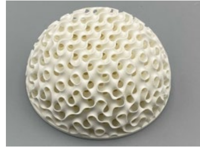
An additively manufactured ceramic GRIN lens produced on the FLUX CORE machine with High Purity Alumina (99.8%) (HP-A 98) resin (Courtesy Tethon 3D)
