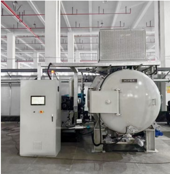
Fig. 10 Large-volume vacuum batch sintering furnaces used in MIM production, with capacities ranging from 1,500 to 3,000 L (Courtesy HIPER/SinterZone)
