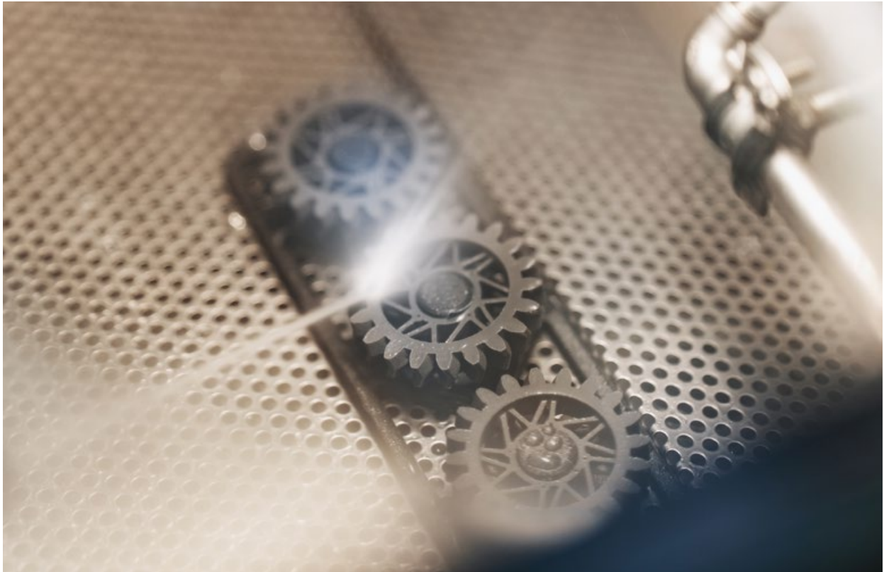
Fig. 4 ColdMetalFusion-produced components undergoing water blasting (Courtesy Headmade Materials)
