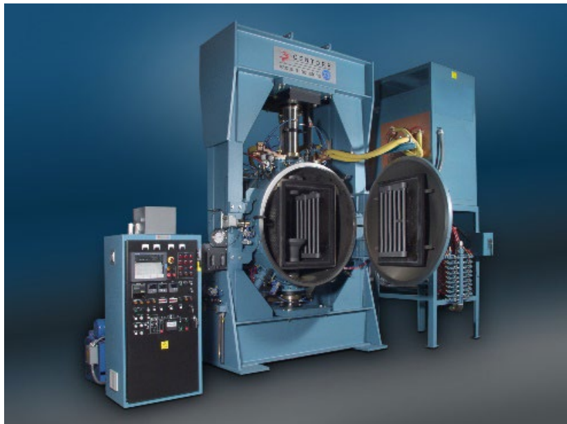
Fig. 13 SiC hot press for producing armour materials (Courtesy Centorr Vacuum Industries)
