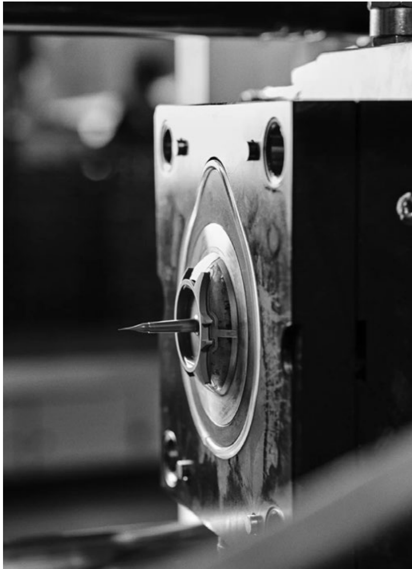
Fig. 6 Celebrating the CIM process: a Chanel promotional image showing a J12 watchcase before removal from the mould (Courtesy Chanel)
