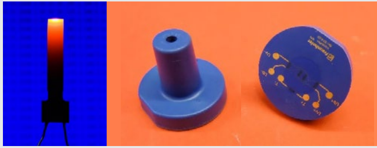
Fig. 2 Left: ceramic glow plug (CIM) [2]. Right: pressure sensor, hybridisation of multilayer technology and CIM [3]
