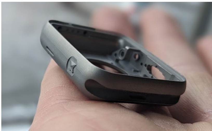
Sintered titanium smart watch housing before surface modification (Courtesy Incus/Element22)
