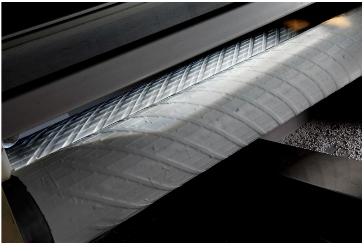
Fig. 2 The most important piece of equipment in feedstock production: the shear roll extruder (Courtesy INMATEC)
