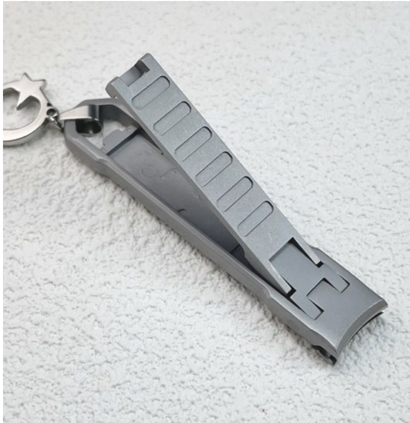
Fig. 7 A foldable stainless steel 420 steel nail clipper manufactured using MIM technology. The powder is produced from the scrap of forged kitchen knife production (Courtesy CHAOYI)
