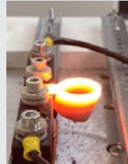
Ceramic heater based on \text{Si}_3\text{N}_4 - \text{MoSi}_2 -mixtures, CerAM FFF [28]
