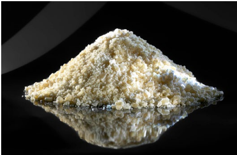
Fig. 4 Embemould wax-based binder for INMAFEED feedstocks (Courtesy INMATEC)
