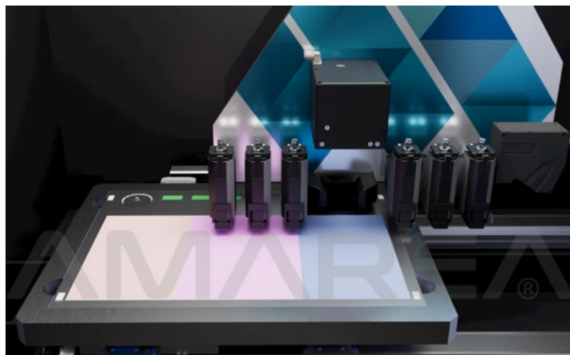
Fig. 11 Preview of AMAREA Technology's series industrial multi-material AM machine based on MMJ with six print heads (left to right), integrated 3D profile sensor (right), and optional laser module (centre)
