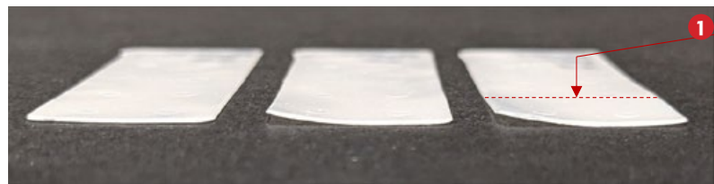
Sintered: 0.3mm / CIM+ / Zirconium Feedstock / 140°C / 1200, 1600, 2000 bar
