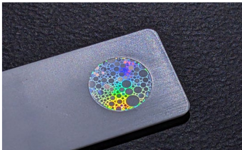
Fig. 1 Optimising the Ceramic Injection Moulding process with variotherm technology delivers improvements in process stability and quality. In relation to the manufacture of holographic structures such as this, significant advances in quality and process capability are achieved (Courtesy iRAP Institute, HEIA-FR/HES-SO, Morphotonix)
