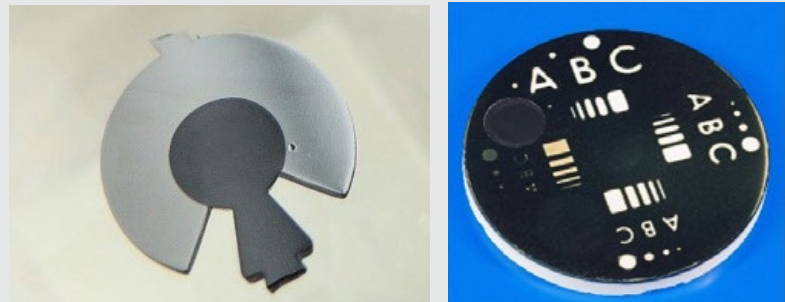
Fig. 4 Left: CIM hardmetal-cermet combination [10], right: jewellery components, In-mould-labeling (tape and CIM) [11]
