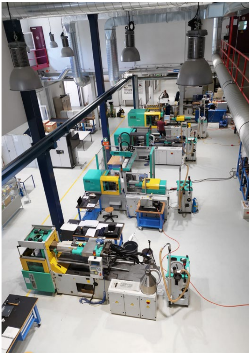
Fig. 2 Laboratory for Plastics and Ceramic Injection Moulding at the Institute for Applied Plastics Research (iRAP) in Fribourg. Beside injection moulding, iRAP is active in compounding and recycling, composite materials, material characterisation, surface treatments and nanotechnology. The institute has specific expertise and equipment for Ceramic Injection Moulding and supports industrial partners in the development of innovative products, processes and solutions (Courtesy HEIA-FR/HES-SO)
