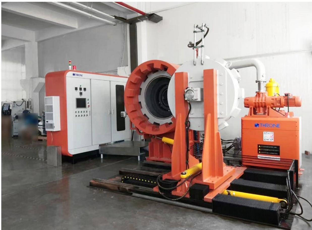
Fig. 5 A high-pressure furnace used for MIM production (Courtesy Throne)
