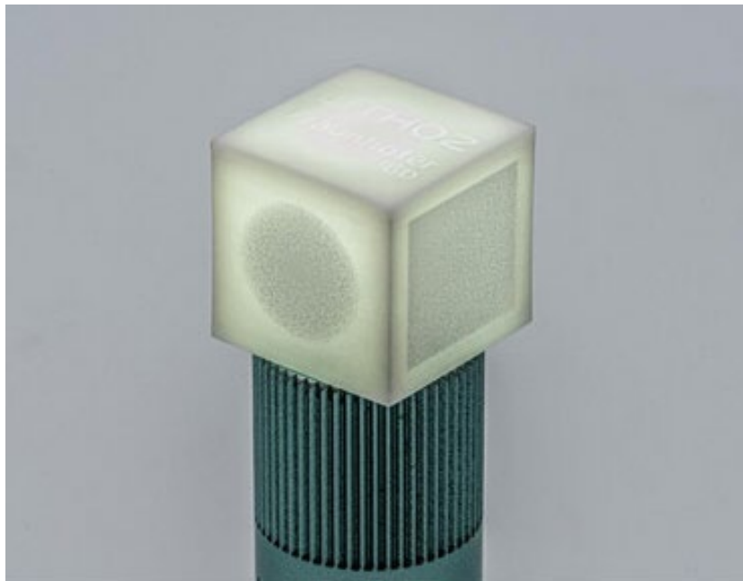
Fig. 7 Alumina component with graded porosity [27]
