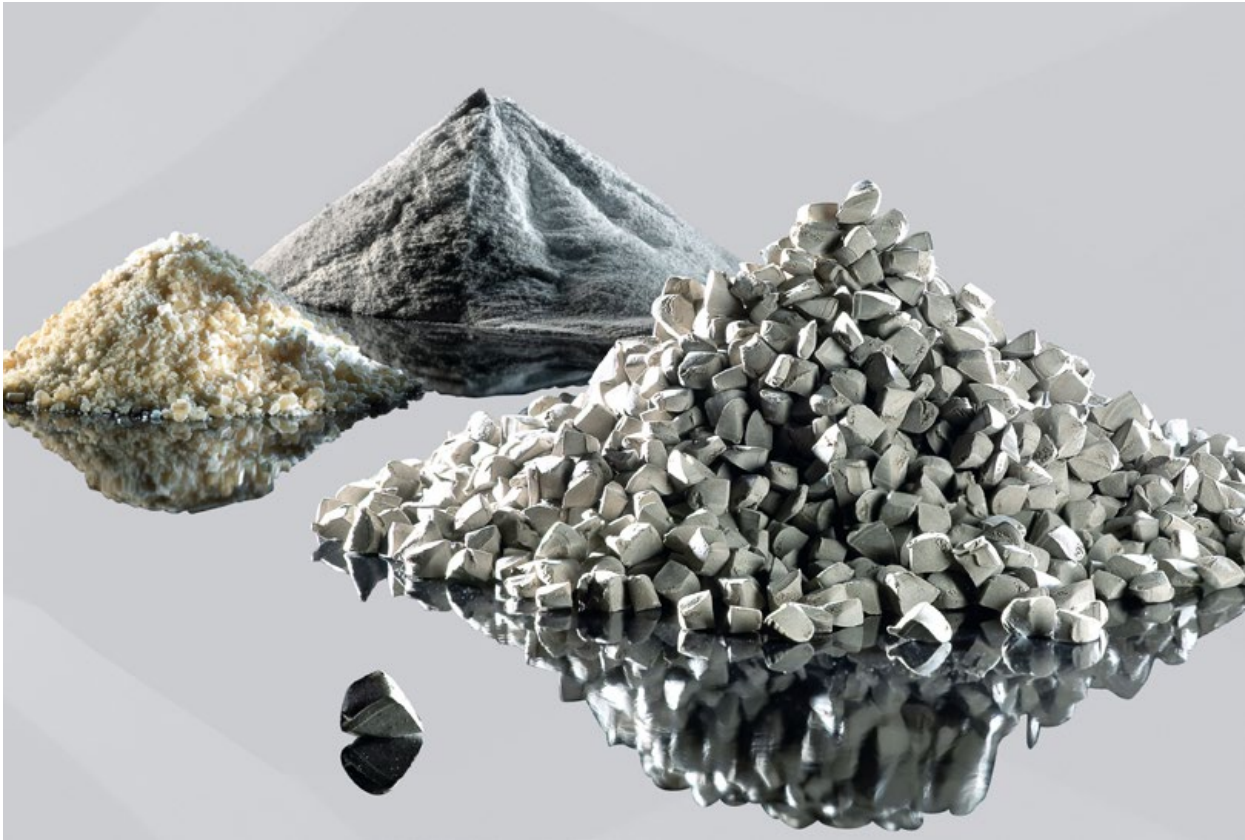
Fig. 5 Binder, powder, and feedstock pellets (Courtesy INMATEC)
