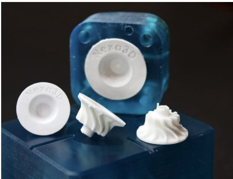
Fig. 10 Additively manufactured tool inserts by Nexa3D which can then be used for low volume CIM - in this case using INMATEC's feedstock (Courtesy Nexa3D)
