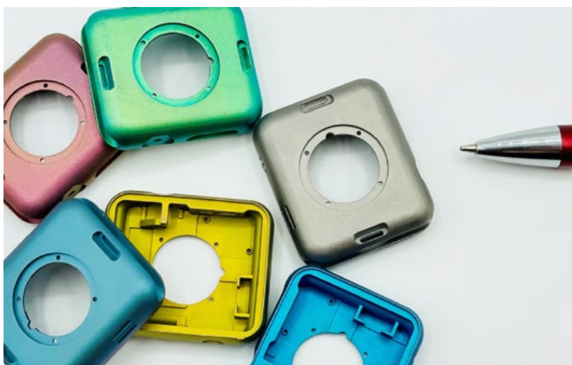
The watch housings undergo a sandblasting stage before being coloured (Courtesy Incus/Element22)
