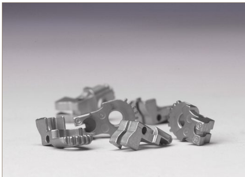
Fig. 7 2011 MPIF award winning 17-PH stainless steel distal channel retainers manufactured by Kinetics. The complex, multi-level part is the main distal-side component of an articulation joint in an articulating mechanical stapler/cutter used in endoscopic surgery
