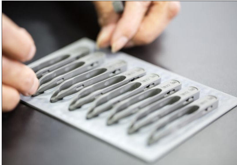
Fig. 4 Green MIM components prior to sintering
