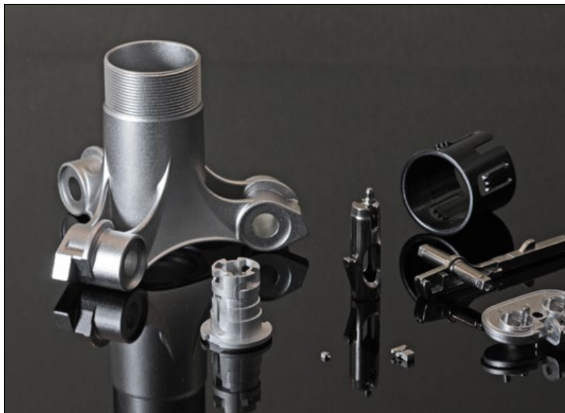
Fig. 1 This selection of EPMA award winning MIM parts not only shows the shape capabilities of the MIM process, but also the variation in part size. Parts shown range from an extremely small 316L eyewear hinge part weighing just 0.028 g to a photographic tripod component weighing just 260 g
