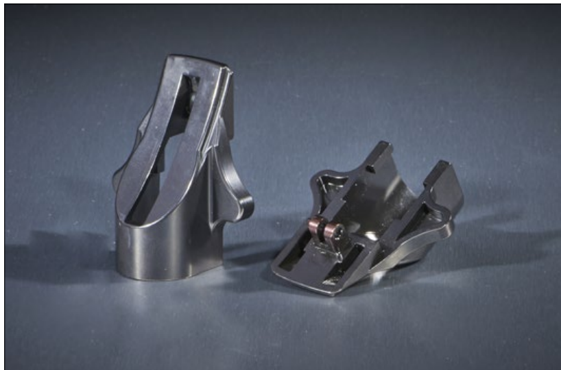
Fig. 5 This 2014 MPIF award winning MIM part was manufactured by Advanced Forming Technology, an ARCMIM Company, and is used in a lock hood for a Smith and Wesson muzzleloading rifle. Manufactured via MIM from 4605 low-alloy steel, the hood's complex geometry presents a challenge in maintaining the large U-shape sufficiently undistorted so that it can be coined into final tolerance. This is accomplished using an 'active' setter made of a feedstock having a similar shrink rate to the hood (Photo courtesy MPIF)
