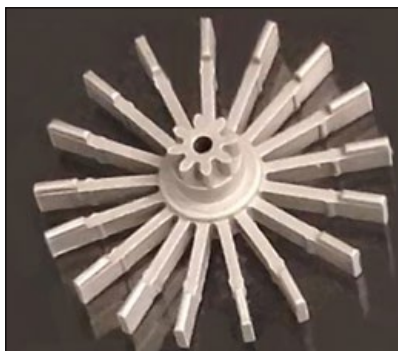
Fig. 8 A MIM sample part produced with the new 6061 feedstock [3]
