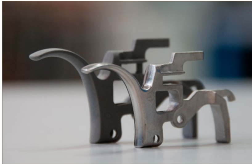
Fig. 4 This MIM titanium trigger is shown in the green and sintered state and was manufactured by Mimest SpA, Trento, Italy
