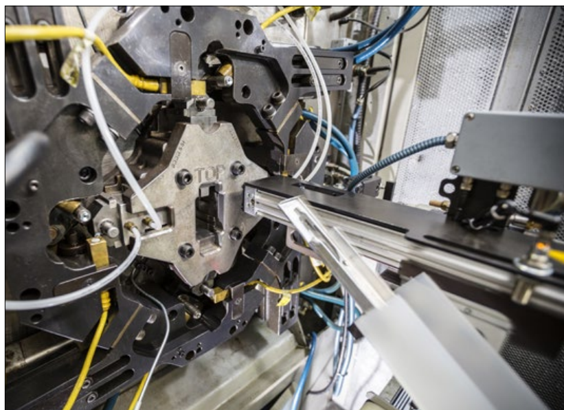
Fig. 1 An A2 injection moulding machine at Dynacast, showing the company's unique multi-slide tooling
