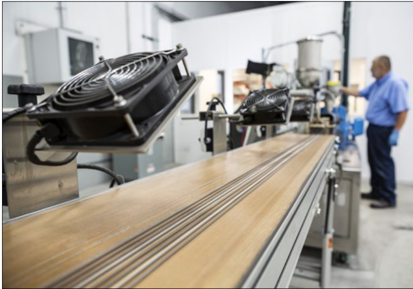
Fig. 2 Extruded MIM feedstock at Dynacast prior to pelletisation
