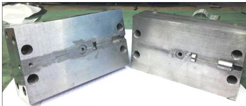
Fig. 9 Injection mould with lost cavity [4]
