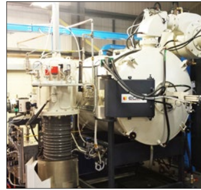
The new ECM Technologies vacuum furnace will be used to process MIM titanium components
