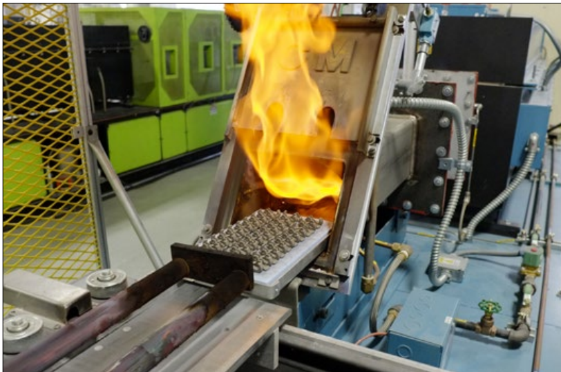
Fig. 3 MIM firearms parts entering a continuous pusher sintering furnace at Megamet Solid Metals Inc, St. Louis, USA
