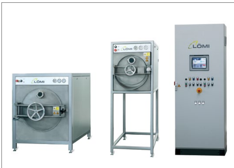
Fig. 4 A modern solvent debinding furnace (left) with a solvent recovery system (centre) and control unit (right) (Courtesy LÖMI)
