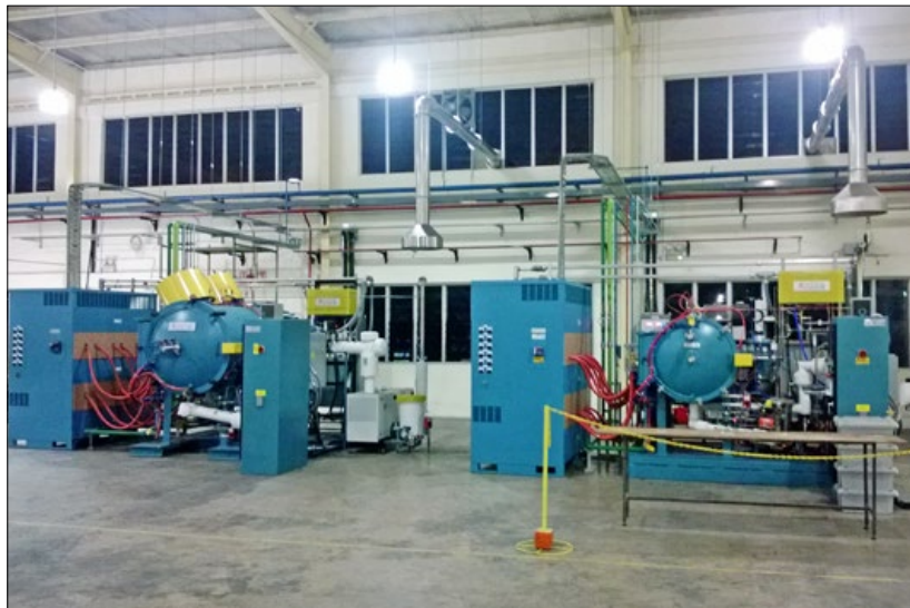
Fig. 5 Centorr Vacuum Industries MIM-Vac furnaces at Dynacast's Singapore MIM operation
