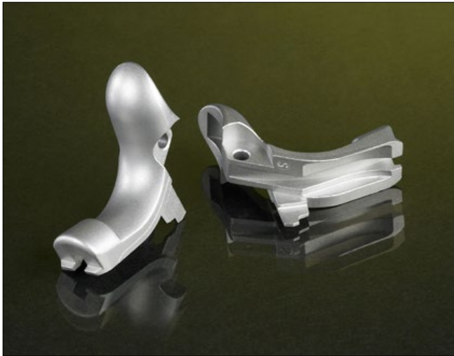
Fig. 8 This 2010 MPIF award winning 17-4 PH stainless steel MIM upswept grip safety was manufactured by Megamet Solid Metals, Inc. and is used in a 1911 45-calibre pistol made by Colt's Manufacturing Company, LLC. The upswept design of the grip safety part, which was traditionally investment cast, would previously require extensive secondary machining. Switching to MIM reduced lead times and provided exceptional cost savings, in addition to increasing production rates and producing a more uniform part. Colt performed a 10,000 cycle test to qualify the part (Photo courtesy MPIF)
