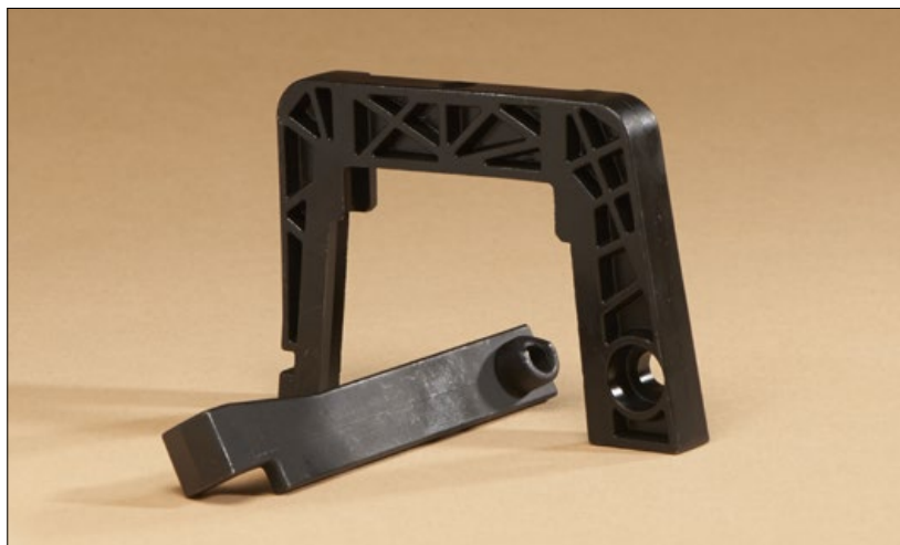
Fig. 10 This 2013 MPIF award winning U-bracket and stop is manufactured by Polymer Technologies and used in a Feedbox Support Improvement Kit (FSIK) for an M249 squad automatic weapon (SAW). The innovative I-beam and webbing design allowed the parts to meet the 32-38 HRC hardness range requirement whilst also saving on weight. Moulded from MIM-17-4 PH stainless steel, the parts have >7.5 g/cm 3 density, 130,000 psi ultimate tensile strength, 106,000 psi yield strength, and 6% elongation (Photo courtesy MPIF)
