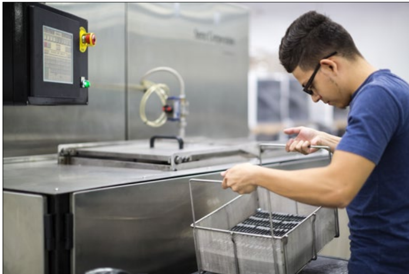
Fig. 3 MIM components loaded in baskets for solvent debinding
