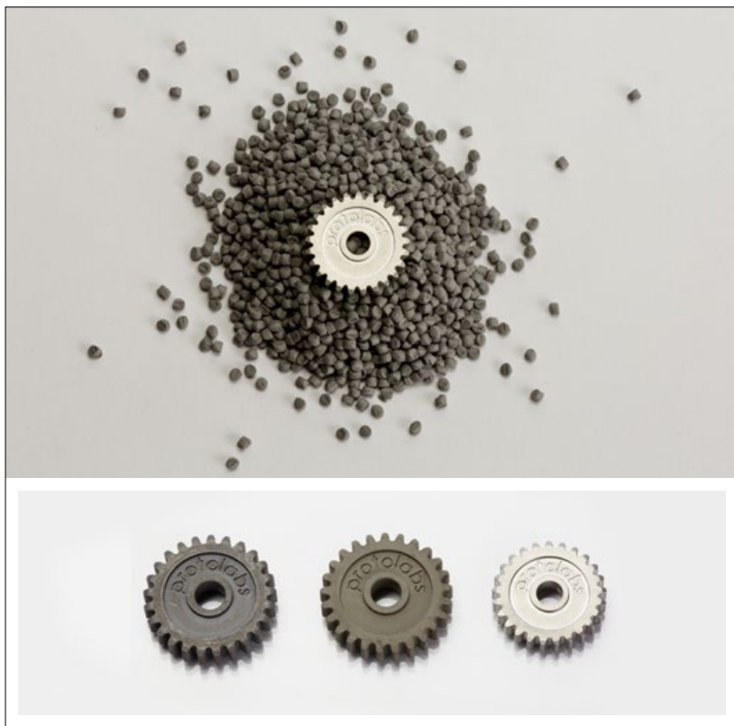
Fig. 2 The top image shows a sintered MIM demonstration part along with granulated MIM feedstock ready for processing. The lower image shows the same part in the as-moulded "green" state (left), in the "brown" state following first stage debinding (centre) and in the as-sintered state (right)
