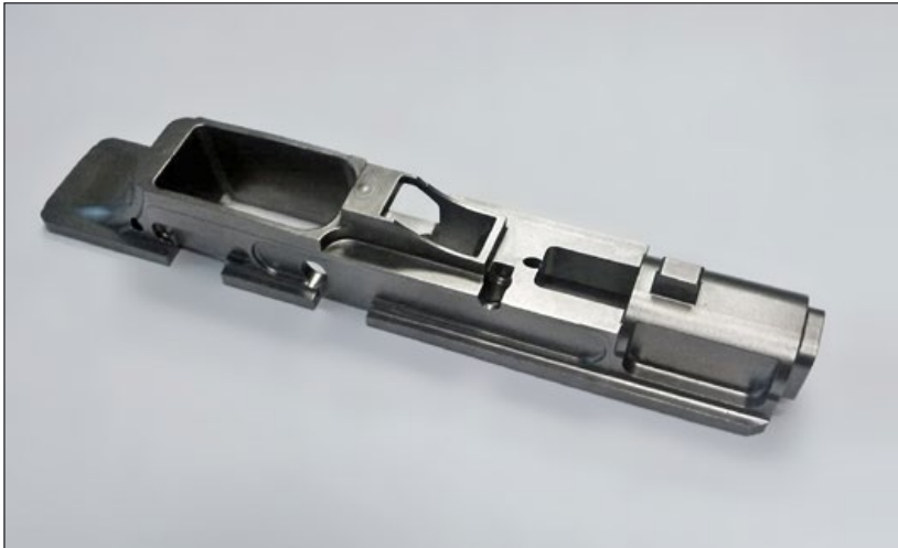
Fig. 11 A MIM underbarrel manufactured by Mimecrisa, Spain, from 8740 heat treatable steel and hardened to 33-37 HRC. The part weighs 168 g and one of the main processing challenges was achieving a flatness of 0.15 mm
