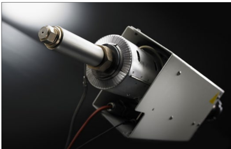
Fig. 3 An elongated PIM nozzle penetrates deep into the mould, enabling sprues to be efficiently shortened (Courtesy Arburg)
