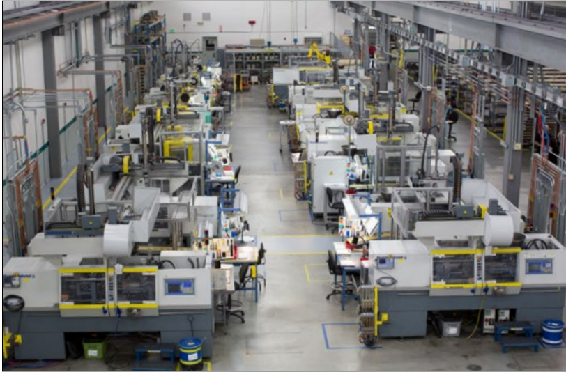
Fig. 2 Injection moulding of MIM parts at Advanced Forming Technology (AFT), an ARCMIM company, in Longmont, Colorado, USA
