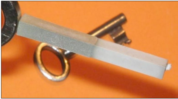
Fig. 14 Fixed connection of metal (stainless steel 430L) and ceramic [ZrO 2 ] materials created by 2C-PIM [5]
