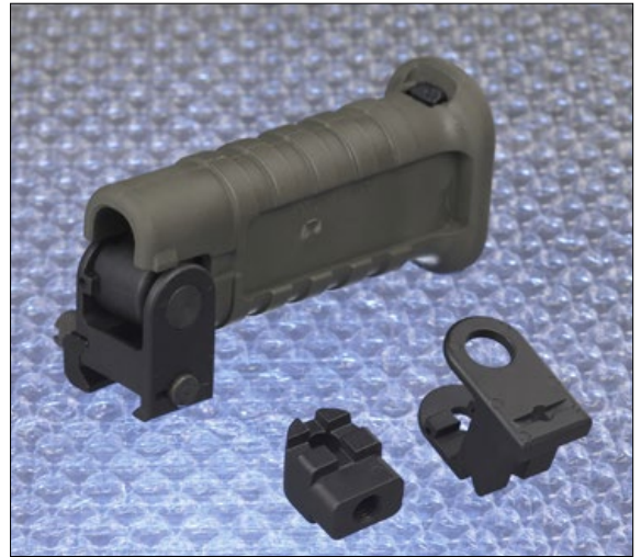
Fig. 9 This 2009 MPIF award winning MIM handle body and yoke was manufactured by Megamet Solid Metals for Colt Canada Corporation. Made from 4140 low-alloy steel, the parts are core components in a folding-front-grip assembly used on modern military rifles. Post-sintering operations included coining, reaming, and tapping. The components are quenched and tempered to a 45-50 Rockwell C hardness range. Parts are supplied to the customer with a manganese phosphate finish (Photo courtesy MPIF)
