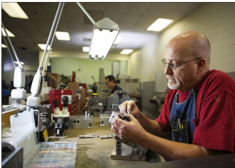
Fig. 6 Maintaining multi-slide MIM tooling at Dynacast
